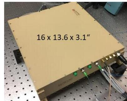
**Figure 1.** Wind-SP High-Power (left) & Low-Power (right) Transceiver Modules which contain the laser & optical components of the lidar except for the T/R telescope.
